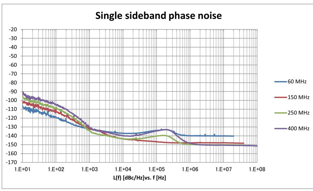
■ 60/150/260/400 MHz, CW, Optimize S/N: On, with MG3710A-002
