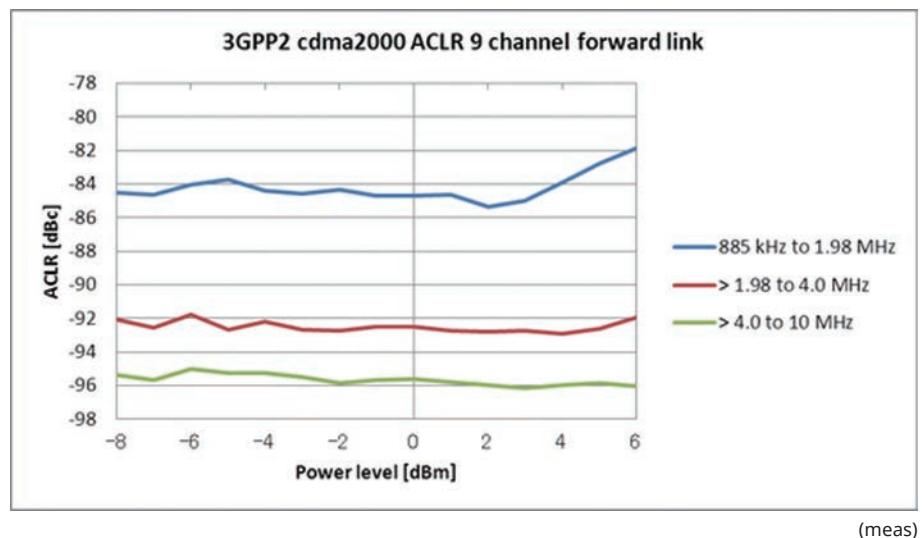
ACLR vs. Power level (with MG3710A-041, Frequency: 850 MHz)
