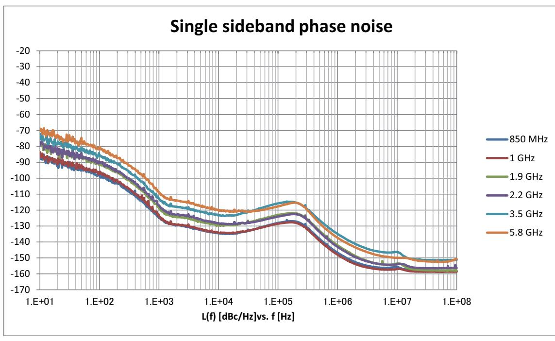
■ 850 MHz, 1/1.9/2.2/3.5/5.8 GHz, Mod = On, with MG3710A-002
